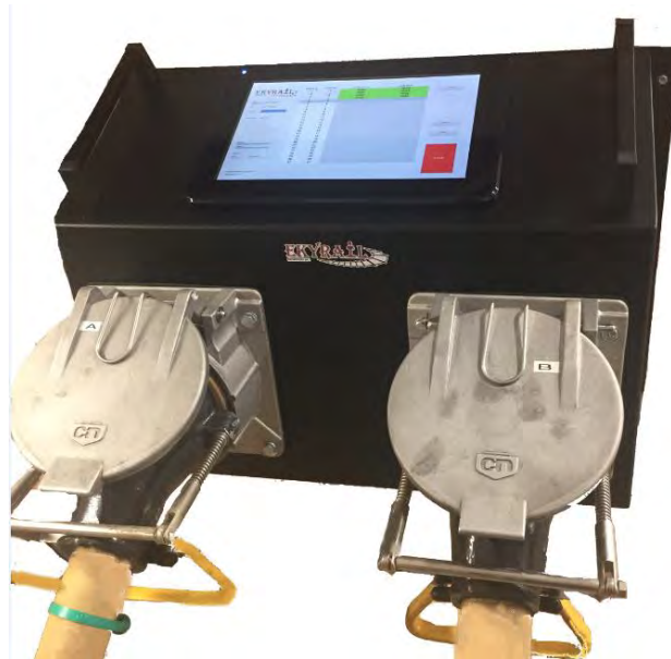
Figure 3 – DUT Cable plugged into Test Ports.
